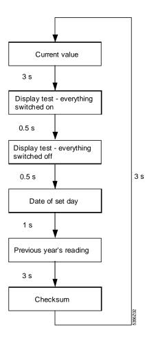
Per default, the heat cost allocator comes with a set day "31.12." and the following display parameters.
